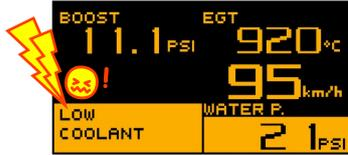
**Little Low Coolant Alarm is very stubborn!** And will override all warnings active in bottom left corner of the display. Its advised that the most important inputs are configured so that when their alarm is active they are not in the bottom left hand corner of the screen.
